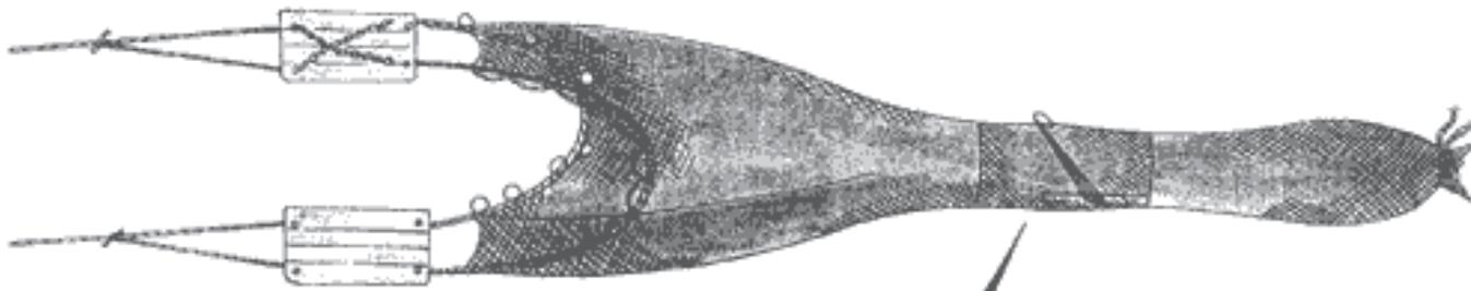
Turtle Excluder Devices are designed to be inserted into trawl fishing nets and allow entrapped sea turtles to easily escape from a trawl net while it is being pulled behind a fishing vessel, as shown in the diagram. The photo below shows a TED frame with the escape flap open.
